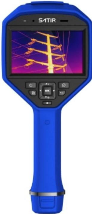
The i-640 is a handheld thermal camera, which come with a Android App, meaning a second person nearby can see what is being surveyed by the person operating the thermal camera. This can be useful if the area being scanned is a small space such as ceiling panels or areas which are restricted to one person.
